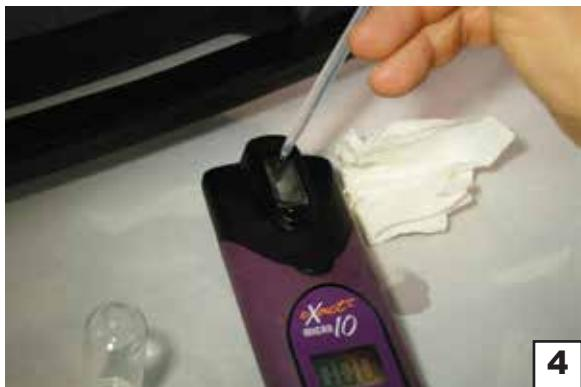
**4.** Discard this first liquid sample followed with a quick shake of the meter to empty the CELL of the remaining water drops.
